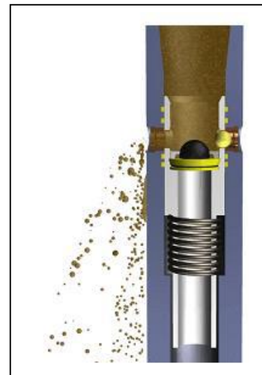
DSI PBL auto-lock feature in action. Draining the string while tripping out of hole.
