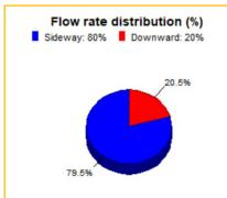
DSI's in-house hydraulics software was utilized to determine the correct ports and dart nozzle sizes to deliver the desired split flow ratios.
