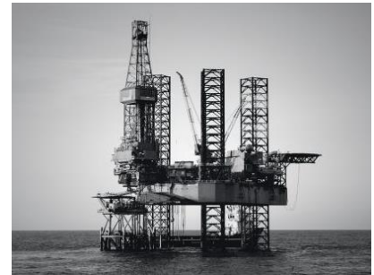
Jack-up rig for drilling in shallow water in Gulf of Mexico.
