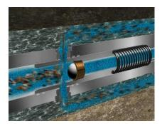
Deployment of aggressive LCM pills thru DSI PBL tool represents a significant cost reduction to drilling companies and operators.
