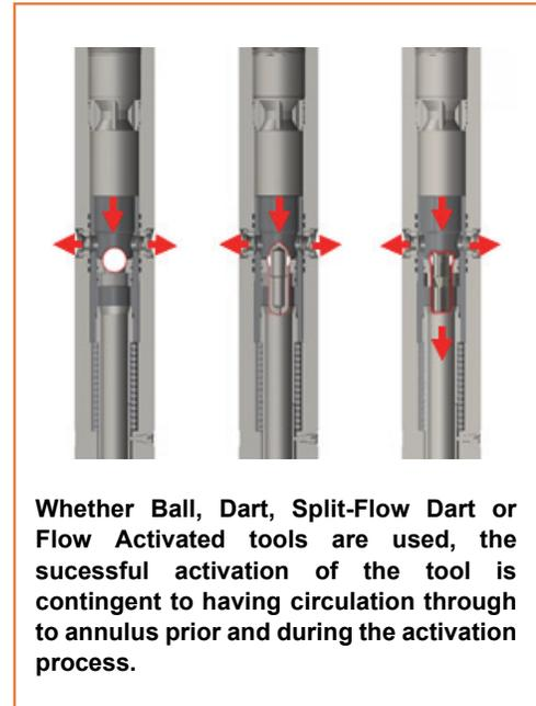
**Whether Ball, Dart, Split-Flow Dart or Flow Activated tools are used, the successful activation of the tool is contingent to having circulation through to annulus prior and during the activation process.**
