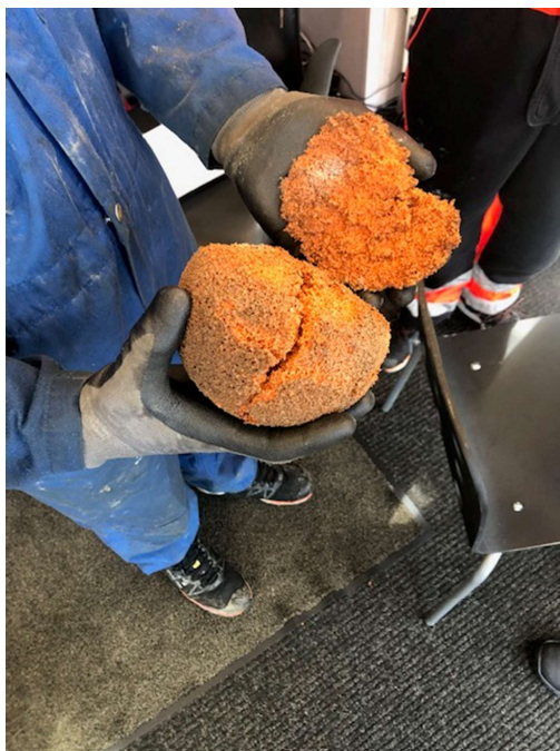
Pic 4. 5" foam ball after passing through PBL ports
