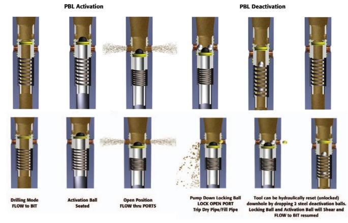
Activating and de-activating of the PBL tool is shown. (Images courtesy of Downhole Devices LLC)
